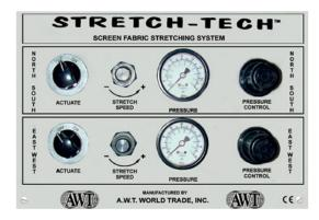
The optional Stretch-Tech™ Auto-Tensioning Module allows fabric to be automatically tensioned in stages, a professional technique recommended by major mesh manufacturers. When stretching screens to the higher Newton levels specified by today's quality-control standards, the mesh must "relax" between stretching intervals to allow the fabric to recover its original physical properties. This procedure eliminates tearing and ensures consistent tension at all points of the screen surface.
