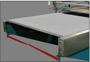
The reciprocating table facilitates loading and, on models with the optional take-off, removing the substrate. The adjustable height locks provide flexible printhead positioning.
