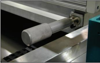
Super micro-registration controls allow for quick, easy setup and precise repeatability of +/-.002"
