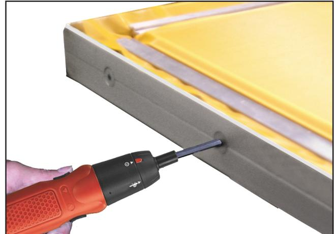
Quick Tension Screws allow you to quickly stretch screens using the included torque screwdriver.
