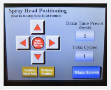
From the convenient control panel, the operator can perform a variety of monitoring and operating functions, including spray head positioning, drain time and total cycles.
